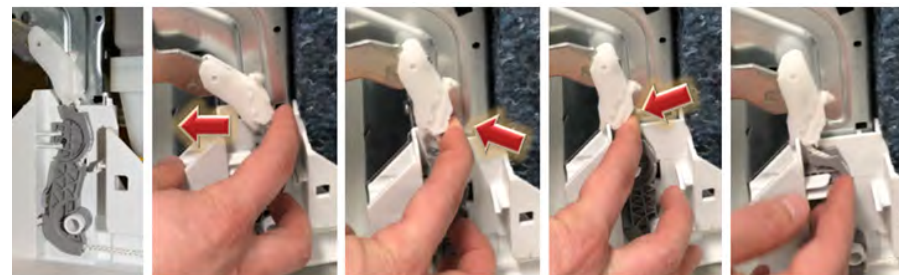
Fig. 86: Parking hinge cords onto base flanges
