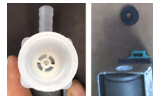
Fig. 33: Water valve with missing filter and loose flow restrictor
