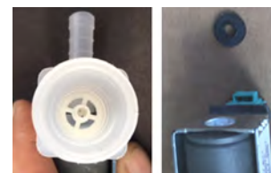
Fig. 92: Water valve with missing filter and loose flow restrictor
