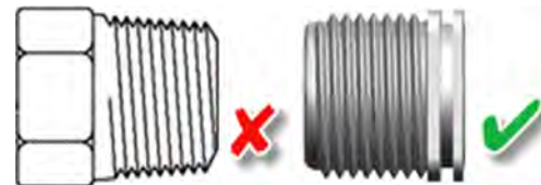
Fig. 91: NPT threads (wrong, left) compared with hose threads (correct, right)
