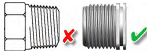
Fig. 32: NPT threads (wrong, left) compared with hose threads (correct, right)
