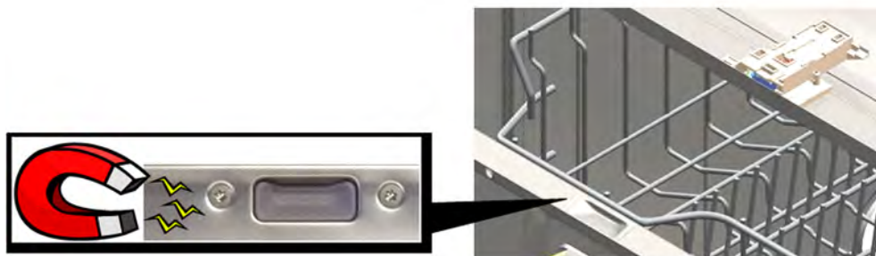
Fig. 78: Checking door latch sensor with a magnet
