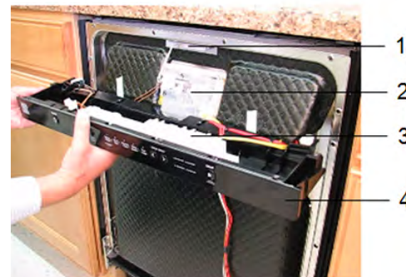
Fig. 76: Parts accessed from the front of dishwashers
