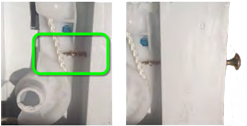
Fig. 56: Consequences of not using supplied toe panel screws
