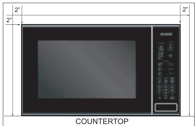
Figure 2-2. 2" Clearance on Sides, Top & at Rear
