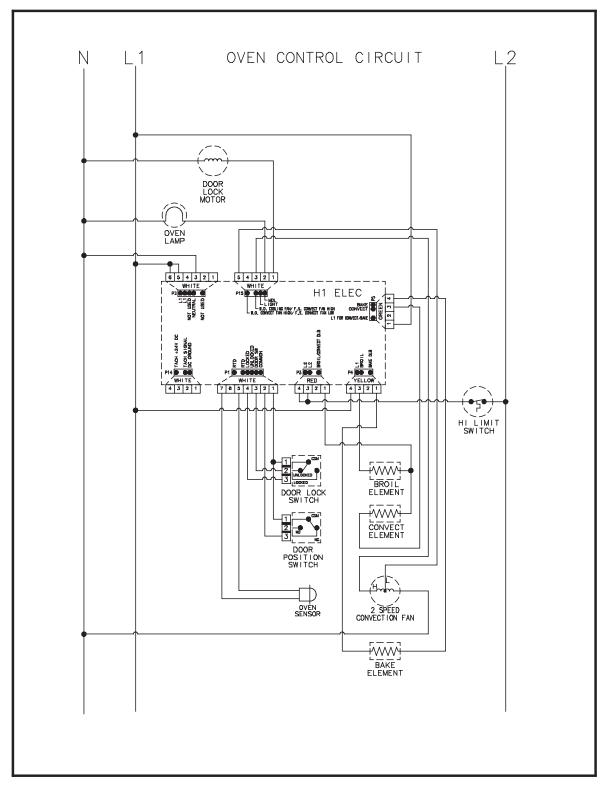
Schematic Diagram (Control Circuits), JER8885QAS Series 15 and later
