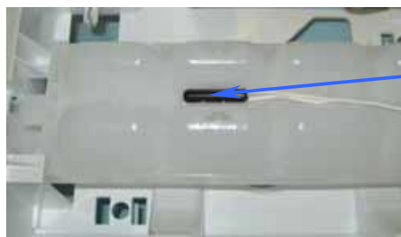
Icemaker sensor located under insulated pad.
