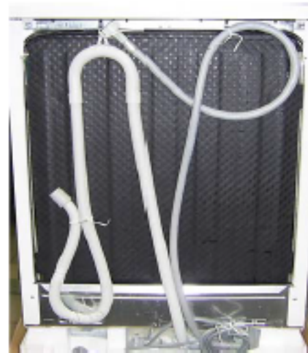
Position of the Drain and Water Supply hoses before disassembling.
