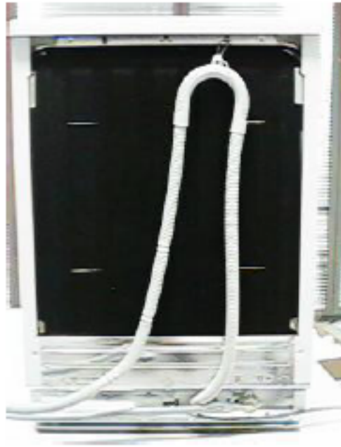
The position of the drain hose during the assembly of the product.
