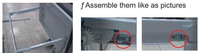
Reinstall the two screws into the guide rails (one from each side).
