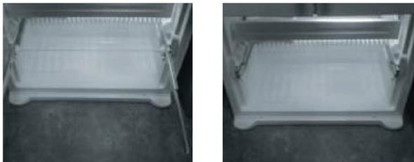
Reinstall the freezer door by inserting the rail tabs into the guide rail.
