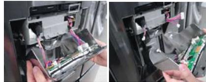
3. Assemble in the reverse order of the disassembly, and assemble while maintaining the horizontality of the Display. After the assembly, to bind 3 Hooks at the top of the Display, lightly hit "tok-tok-tok" with fist.
