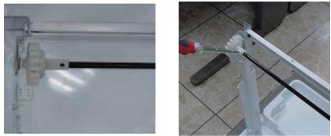
The rail system will align itself by pushing the rails all the way into the freezer section. Pull the rails back out to full extension.
