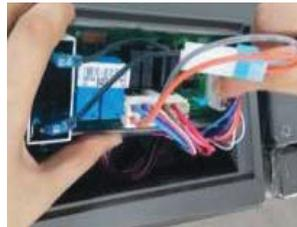
3. Connect the capacitor housing.
