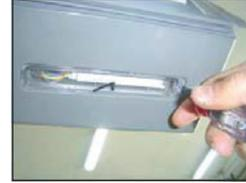
4. Remove the LED assembly from connector.
