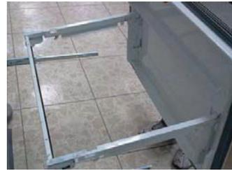
Step 5) Remove only 1 screw of gearice, and disassemble the bar and gearice
