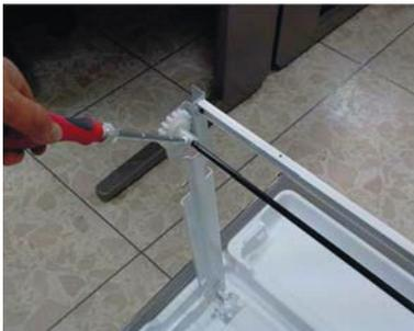
Step 6) Remove 2 screws of both side of supporter covers tv and disassemble the supporter cover tv.
