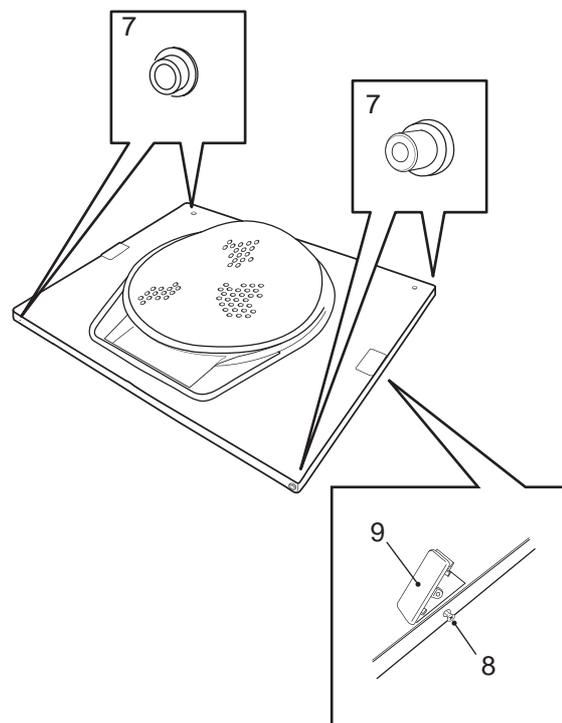
13. Remove the screw that is securing the front panel at the bottom edge of the side where the hinge will be installed.
