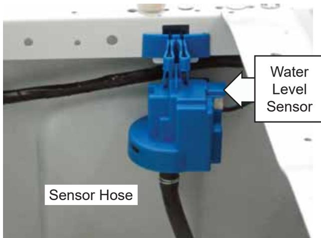
The frequency is monitored by the Main Board, which turns off the water valves when the desired water level is achieved.
