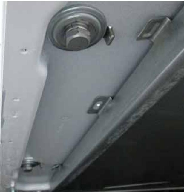
3. Lean the washer back to access and remove the 13-mm hex-head bolt from the bottom of the washer that secures the damper to the chassis.
