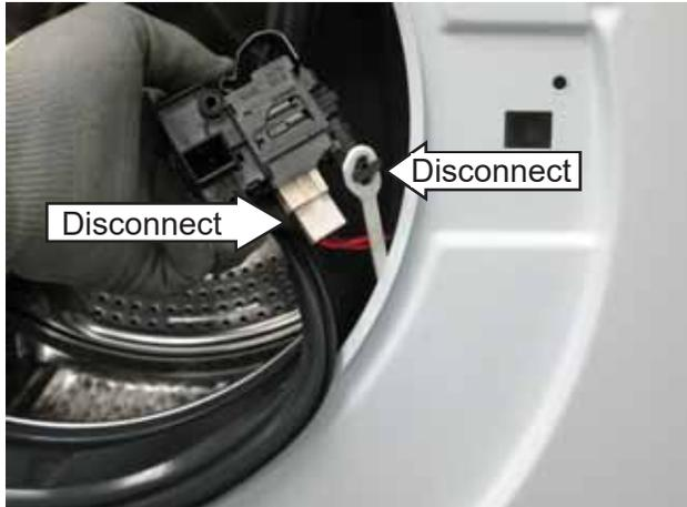
**NOTE:** The door latch is solenoid activated. It can remain locked after the power is removed.
