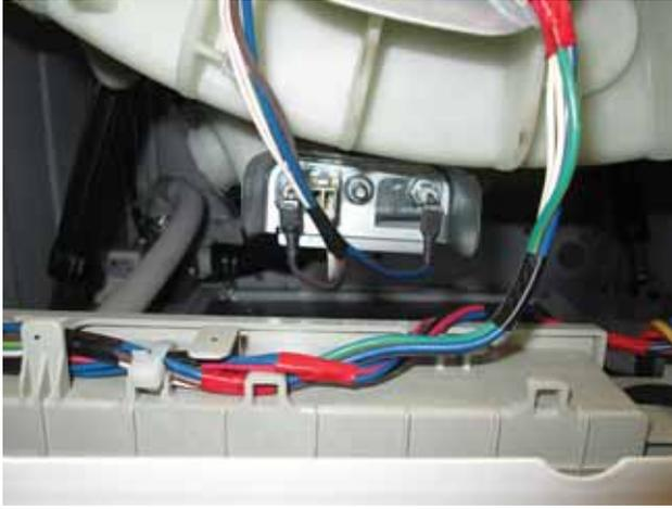
5. Unclip four clips that secure the board access cover to the main board.
