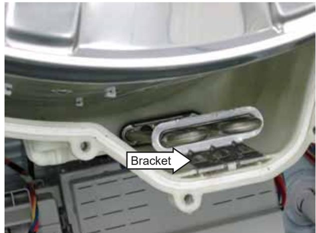
1. Seat the heater assembly in the tub opening.
