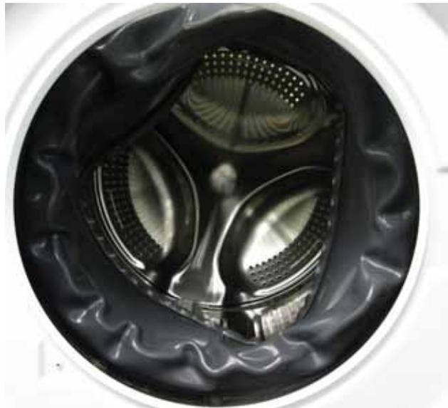
5. Reinstall the inner clamp into the groove so that the clamp adjuster is positioned approximately at the 11 o'clock position.
