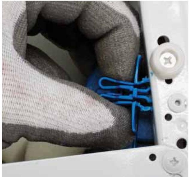
5. Disconnect the pressure tube and harness connector from the sensor.
