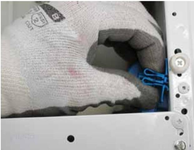
4. Pull the sensor forward to release the rear tab from the opening.
