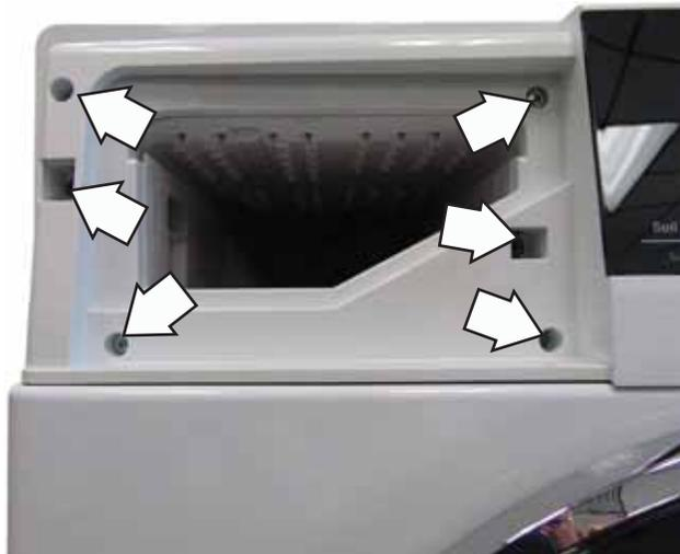
4. Pull the control panel out slightly and raise the left side of the control panel upwards. This will disengage the top left side tab.
