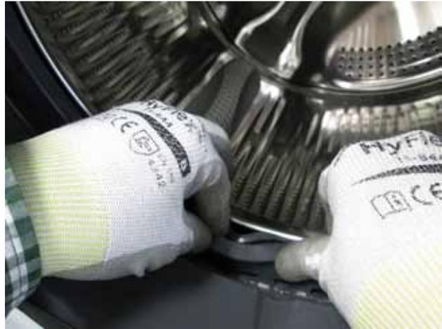
4. Fold the gasket toward the inside of the basket to make it easier to install the inner clamp.
