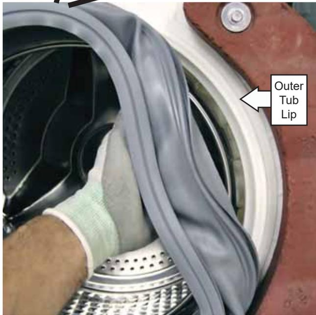
2. Ensure that the gasket is securely seated over the tub lip. It is tight, but this can be done without removing the front counterweights.
