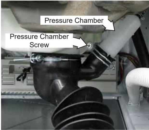
**NOTE:** The pressure chamber is replaceable by removing one screw and then sliding the chamber up to disengage it from the tub.
