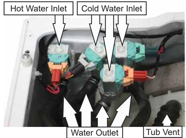
7. Remove the two Phillips-head screws that attach the valve to the cabinet.
