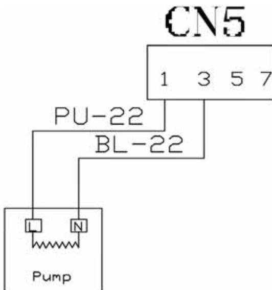
Operation of the drain pump can be checked by using Service Test mode t07 (see the **Service Mode Test** in the Diagnostics section of this guide.)
