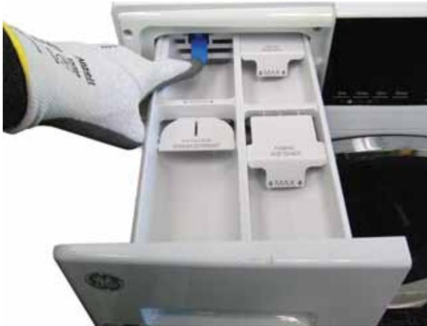
3. Remove the six Phillips-head screws from the control panel dispenser recess.
