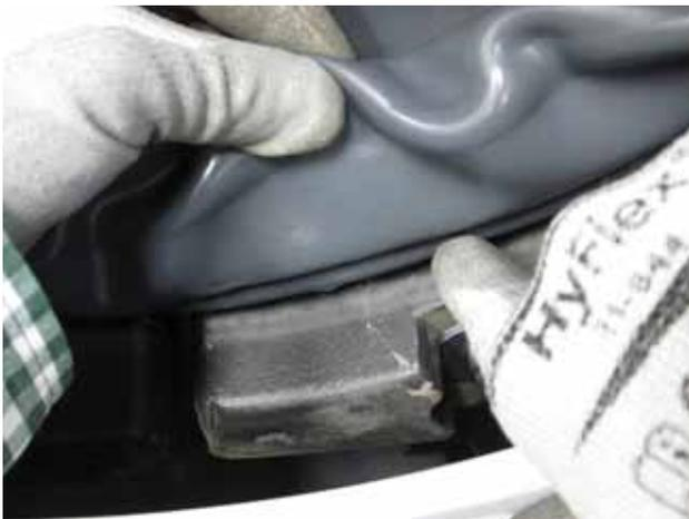
3. Ensure that the gasket does not rub the basket by rotating the basket. If it rubs the basket, make adjustments as needed before installing the inner clamp.
