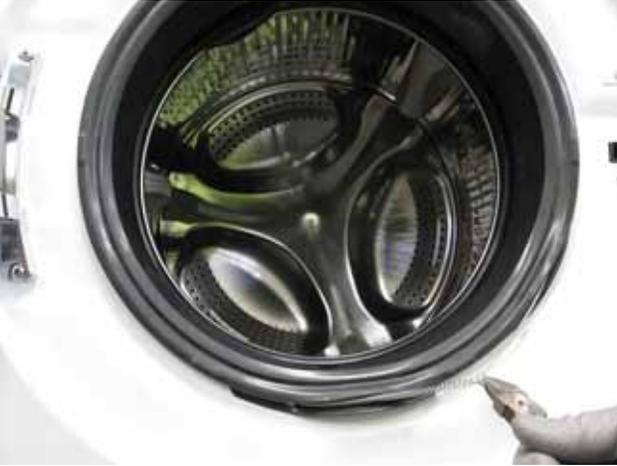
9. Again, ensure the gasket is still seated flat against the front panel. If not, make necessary adjustments.
