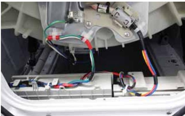
4. Remove the rotor and stator, taking care not to damage the stator harness connections (see **Motor Assembly Removal**, in the **Drive System** section of this service guide, under **Motor Assembly**).
