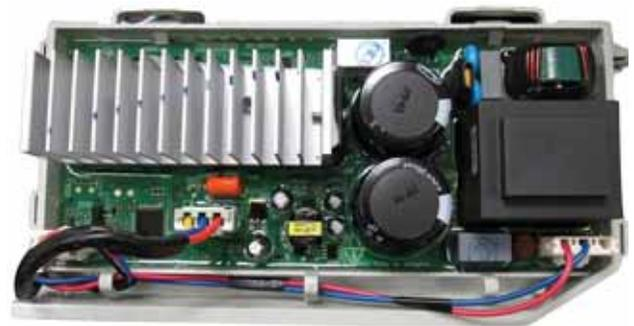
4. Disconnect the harness from the inverter board.
