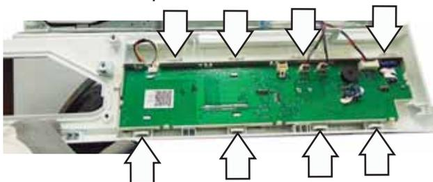
4. Remove the UI from the control panel carefully as to not damage the harness to the Sensor Touch Board.
