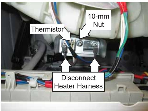
5. Loosen the 10-mm hex-nut until it is flush with the end of the stud.
