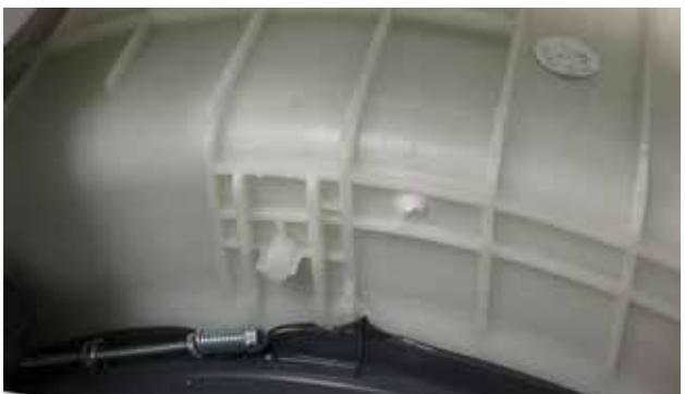
6. Reinstall the gasket over the lip of the front panel ensuring it is flat against the front panel.
